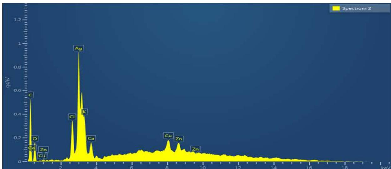
*Fig 6 :EPAX analysis of silver nanoparticle synthesized from dried rhizomes of Z.officinale*
