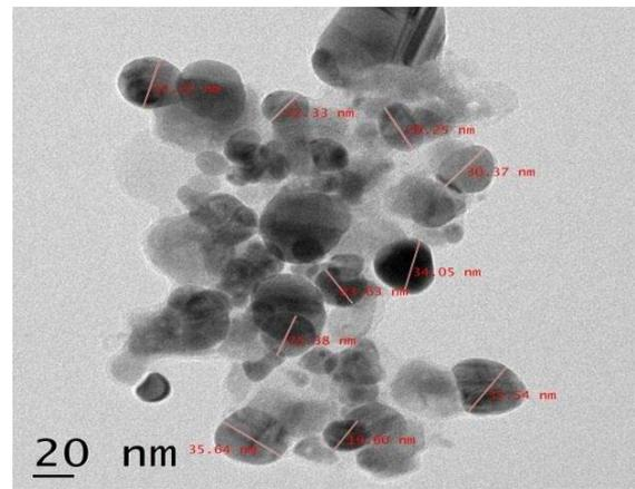
*Fig- 4 a & b : TEM analysis of gold nanoparticle synthesized from fresh [a] and dried [b] rhizomes of Zofficinale*
