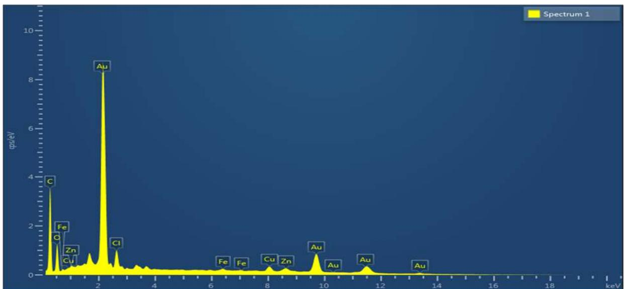
*Fig 8 : EPAX analysis of gold nanoparticle synthesized from dried rhizomes of Z.officinale*
