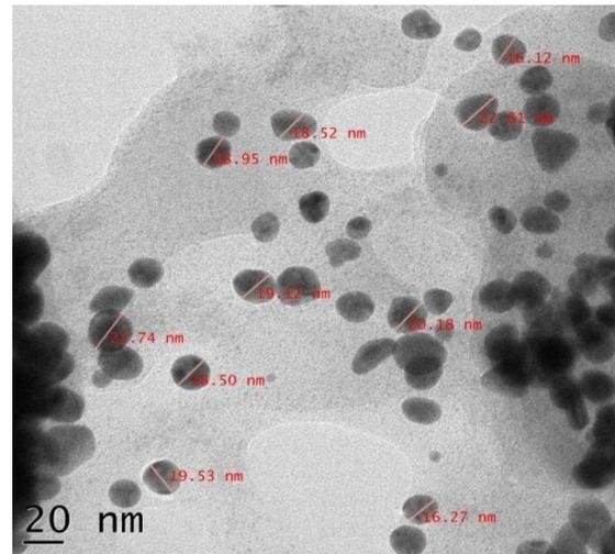
*Fig 5:EPAX analysis of silver nanoparticle synthesized from fresh rhizomes of Z.officinale*
