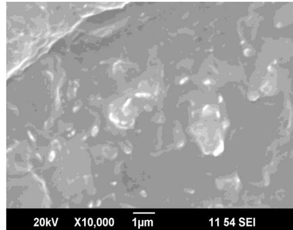
*Fig 2a & b : SEM photos of gold nanoparticle synthesized from fresh[a] and dried [b] rhizomes of Z.officinale*
